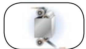
In-line calendering process to achieve surface smoothness on the order of angstroms.
